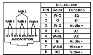
NOTE: These devices is reversible, BNC connector = RJ-45 PAIR4: VIDEO
